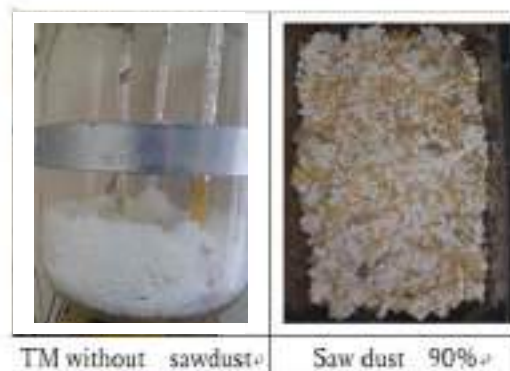
Figure.2 The agglomeration of TM after charging process with and without sawdust.
